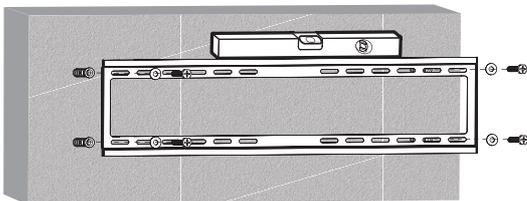
Install the wall plate to the Solid wall or Double Stud wall
