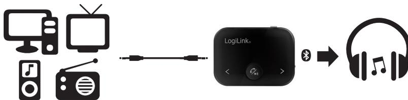
Enables to send audio through BT0050 to the remote device.
