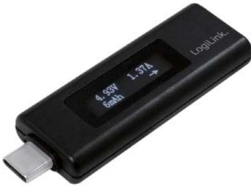
Protect your USB-C™ devices effectively by real-time monitoring the charging performance of the USB-C™ port when charging/utilizing.
