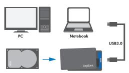
install the SATA HDD/SSD and connect to PC
